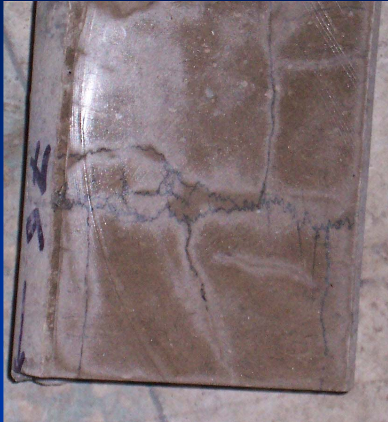
Stylolites, + associated steep tension gashes, and fine veins
